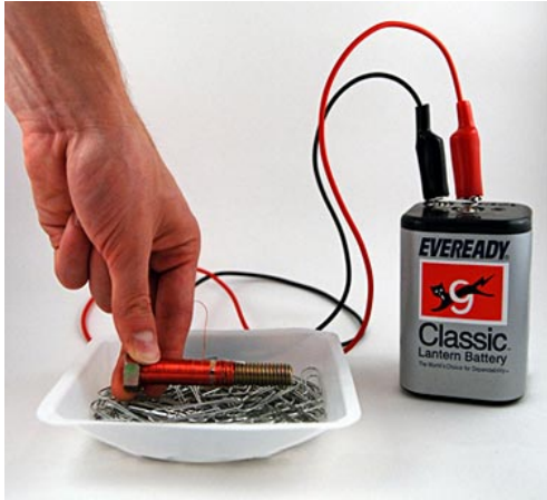
Figure 3. After connecting the alligator clip leads to the battery and wire on the coil, the electromagnet will be energized. Lower the electromagnet into the container of paper clips so that the long part of the electromagnet touches the paper clips.
