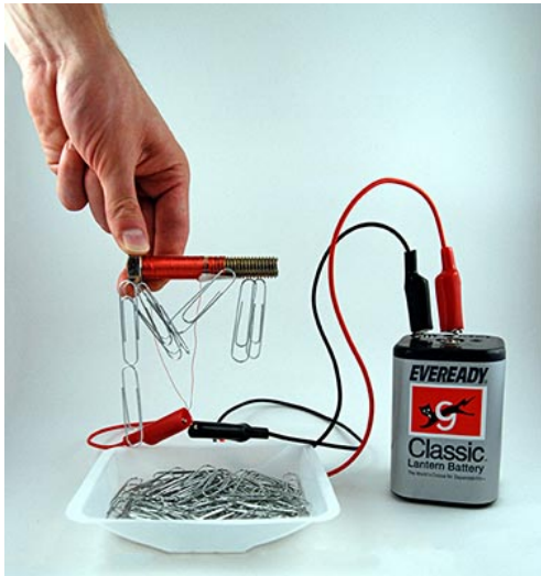
Figure 4. Once you have touched the electromagnet to the paper clips, lift the electromagnet up. Some of the paper clips will stick to the electromagnet. Move the electromagnet away from the container (so that the paper clips will not fall back into the container) and then disconnect the coil from the battery.
