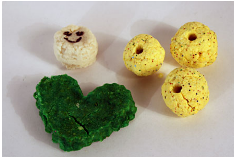
Figure 6. Students can mold and decorate the casein plastic within an hour of making it. It will take at least 48 hours to dry completely.
