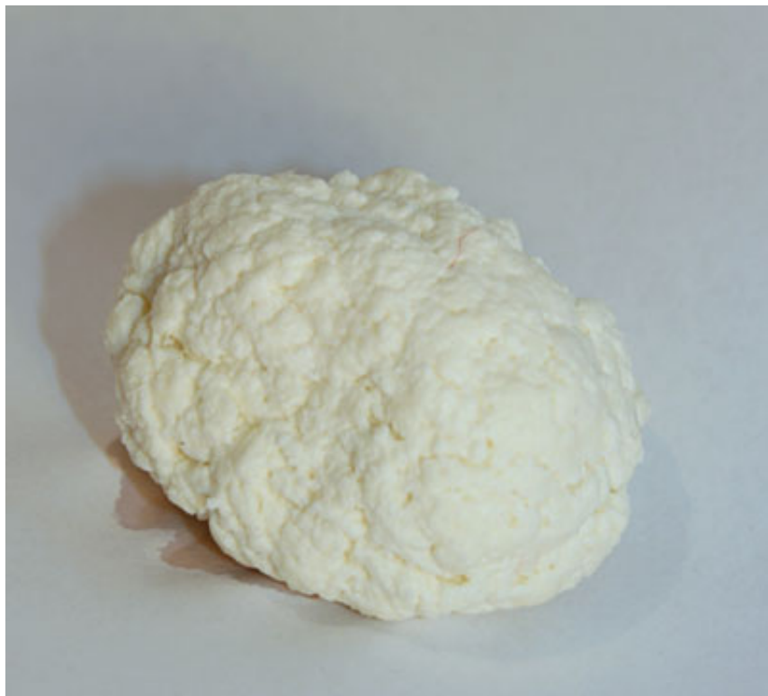
Figure 5. Direct students to press down on the curds with the paper towels to soak up all of the extra liquid. Students should then knead the curds together to make a ball of dough, which is the casein plastic.
