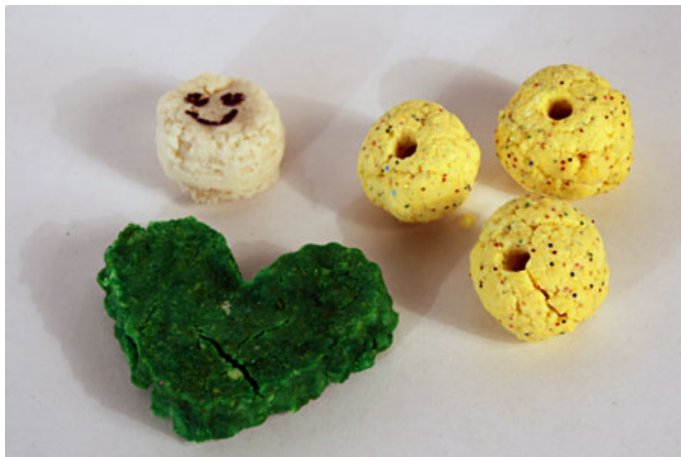
Figure 3. You can mold and decorate the casein plastic into shapes such as these for about an hour after making it. It will take at least 48 hours to completely dry.
