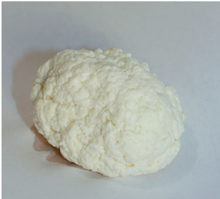
Figure 2. Press down on the curds with the paper towels to soak up all of the extra liquid. Push the curds together to make a small ball, as shown here. This is the casein plastic.
