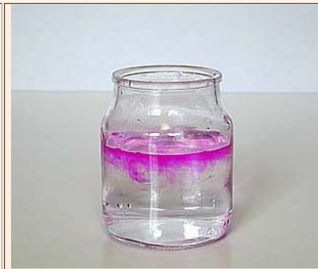
Figure 18 - By adding vinegar, the solution becomes again colorless. The picture illustrates the change in progress.
