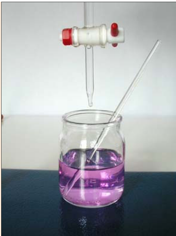
Figure 20 - As soon the liquid in the beaker changes color, stop the dropping.
