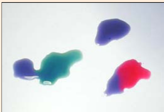
Figure 9 - Red cabbage juice mixed with baking soda (left) and with vinegar (right). On the top, a drop of unmixed juice.
