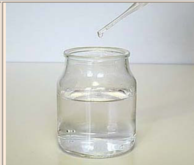
Figure 16 - Add 3 drops of phenolphthalein to 100 ml of water. You will obtain a colorless solution.
