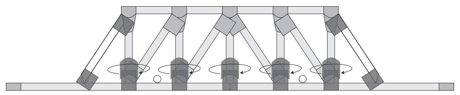
Add top cross supports, using the 5 remaining cross supports from step 3. Lay the bridge bottom-down on the blueprint below (this is a **top-down** view) and tape the 5 cross supports to the sides of the bridge, as shown by the white placeholders, below. The cross supports go above each of the vertical supports.
