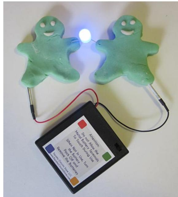
Figure 6. The *shape* of the play dough pieces does not matter; as long as there is a closed circuit for electricity to flow (and no short circuit), the LED will still light up.
