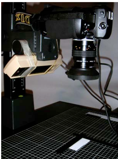
Figure 1: Setup for digital photography of a TLC plate. The camera and UV lamp were attached to a stand to insure that they were always the same distance from the plate.
