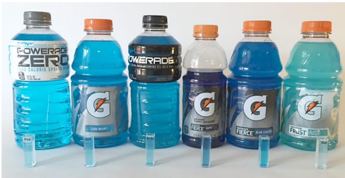
**Figure 7.** Several sports drink samples with unknown concentrations of Blue 1 prepared for measurement on the spectrophotometer.
