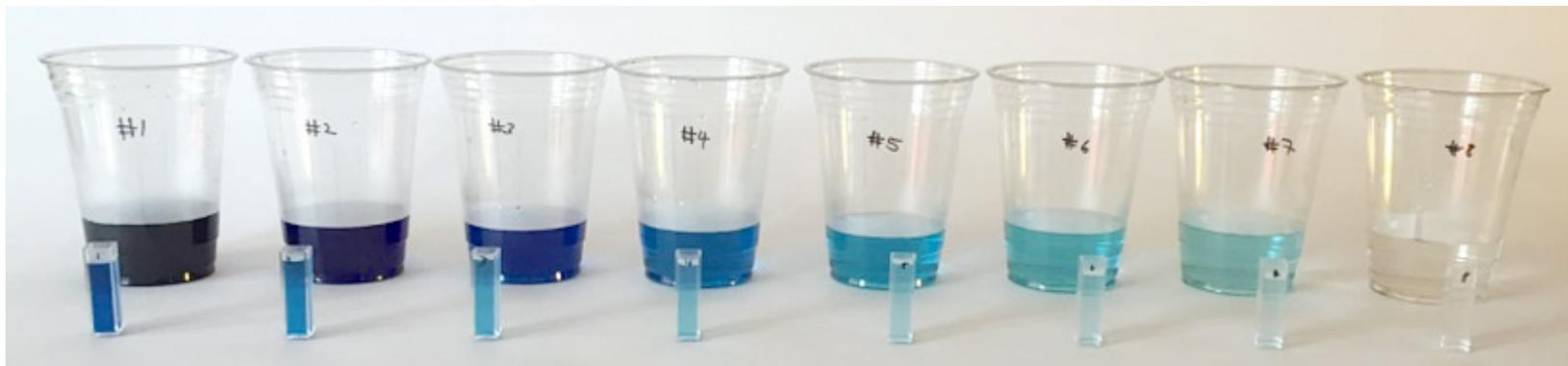
**Figure 5.** Standard solutions of Blue 1 for creating the calibration curve.
