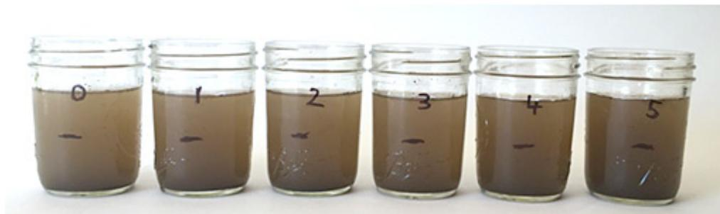
**Figure 8.** Turbid water samples before adding different amounts of flocculant (alum). Note that although this image shows glass Mason jars, you can also use plastic cups for your experiment.
