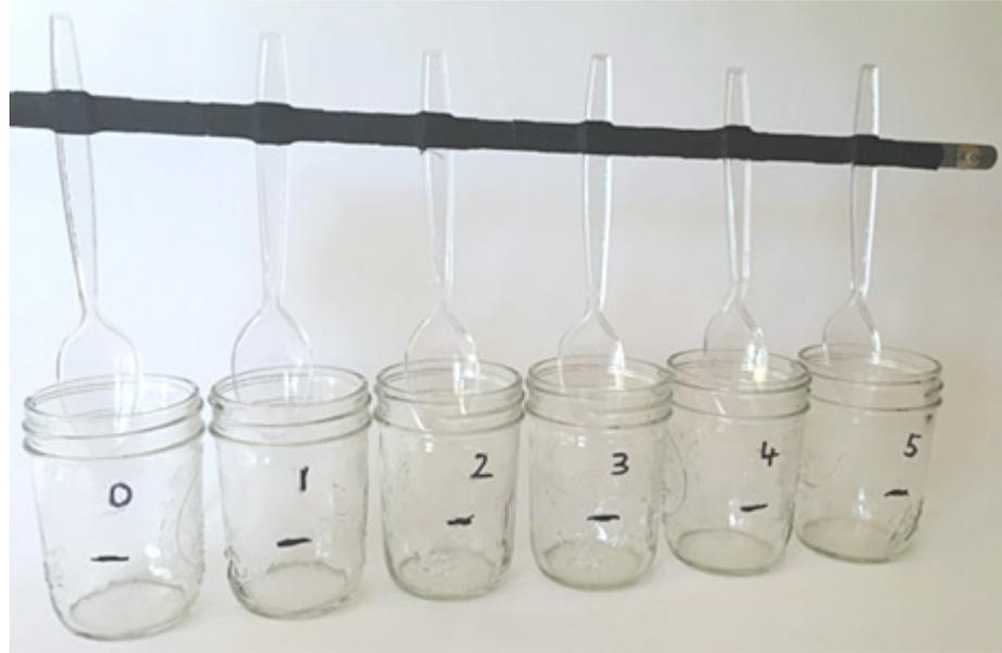
**Figure 7.** Stirring device that allows for simultaneous stirring of six sample solutions. Note that this image shows glass Mason jars, but you can also do the experiment in plastic cups.
