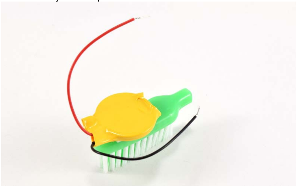
7. Battery attached to toothbrush.
