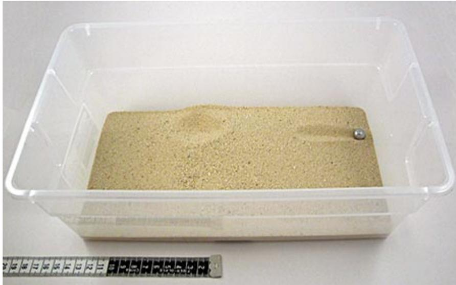
**Figure 3.** In this case, the launched ball bearing landed in the crater at left, then bounced and slid to where it finally stopped at the right side of the box. The tape measure is positioned to start measuring from the circular crater at left—the place where the ball bearing first hit the sand.
