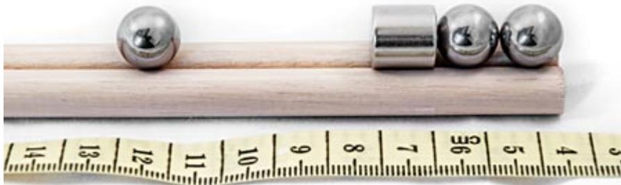
**Figure 2.** A one-stage Gauss rifle. Note the two ball bearings touching the magnet stage at the end of the slide (as described in step 4) and the single ball bearing (the starter ball) 5 cm behind the magnet stage (as described in step 6).
