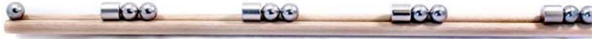
Figure 5. A four-stage Gauss rifle with the "starter" ball bearing 5 cm to the left of the fourth stage. A two-stage launcher has two magnet stages, with the "starter" ball bearing 5 cm from the second stage. Similarly, a three-stage launcher has three magnet stages, with the "starter" ball bearing 5 cm from the third stage. In each case, the magnet stages are 10 cm apart from one another.
