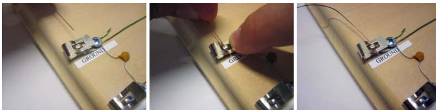
Figure 16. To connect a wire to a Fahnestock clip, first press down on the tab of the clip with your finger. Use your other hand to thread the end of the wire through the clip, as pictured, then release the tab.
