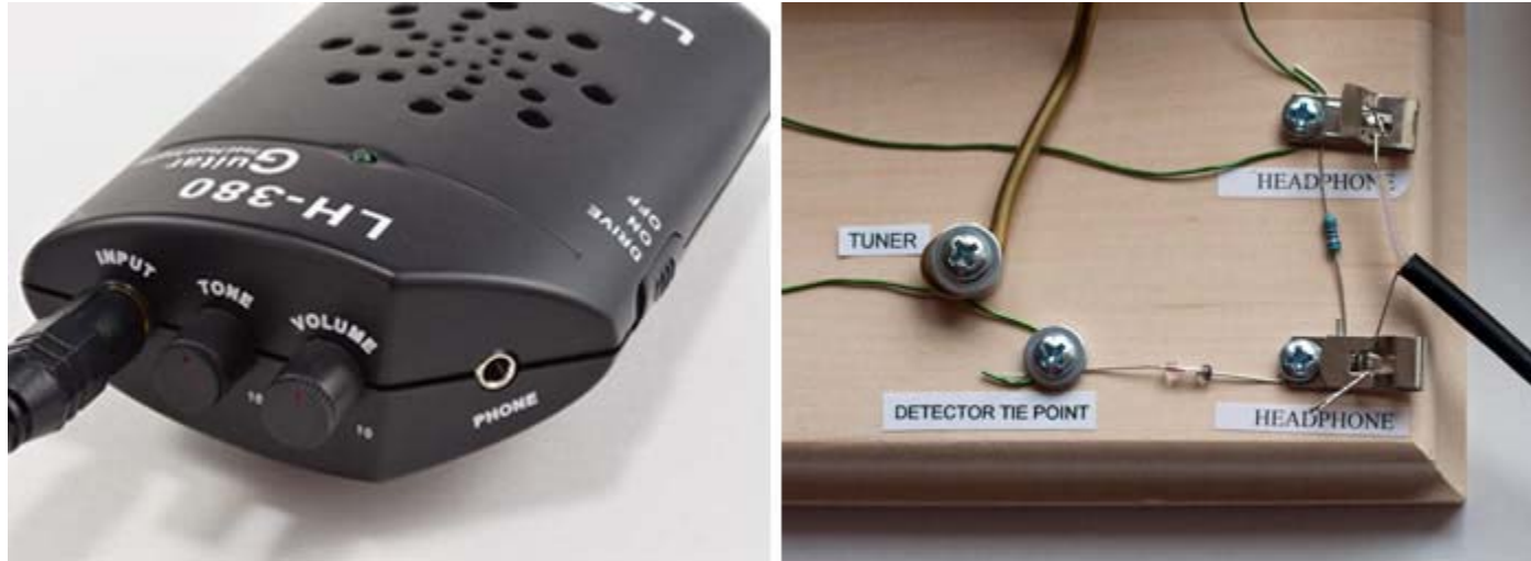
Figure 18. Attach the split ends of your audio cable to the two "HEADPHONE" Fahnestock clips, and plug the other end into the audio amplifier's "Input" jack.
