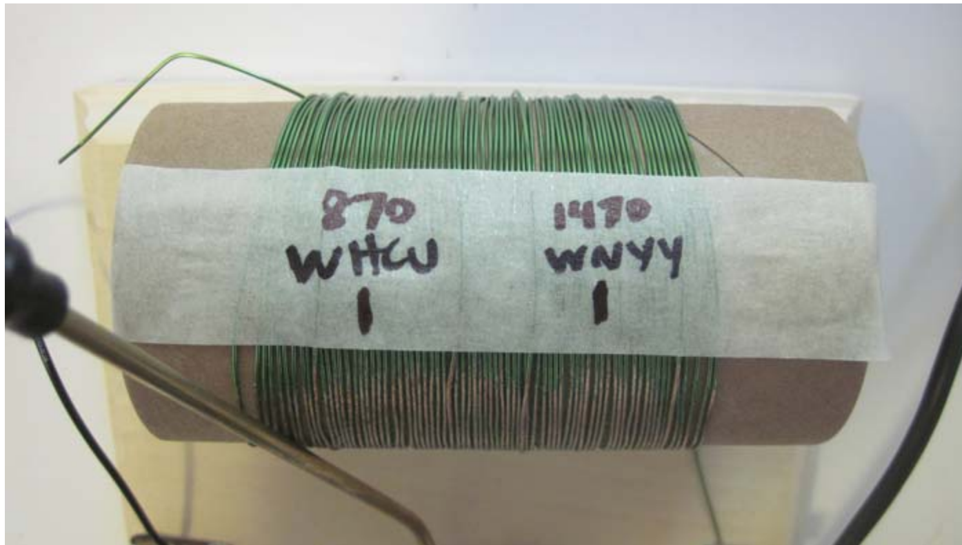
Figure 21. Use a strip of masking tape and a permanent marker to help you identify stations more easily on your coil.
