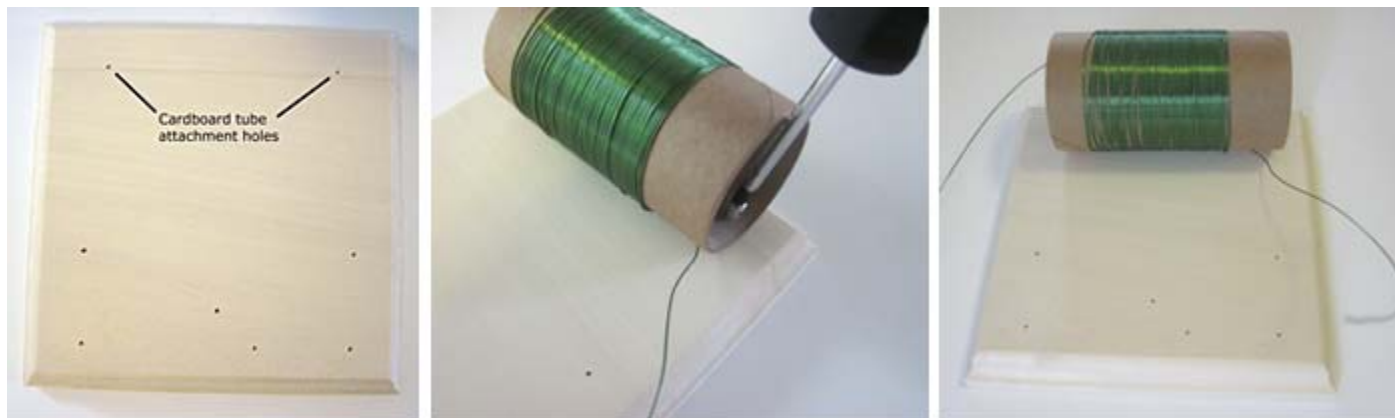
Figure 6. A diagram of Attach the cardboard tube to the wooden baseboard. Be sure to use the correct holes, as labeled in the figure.
