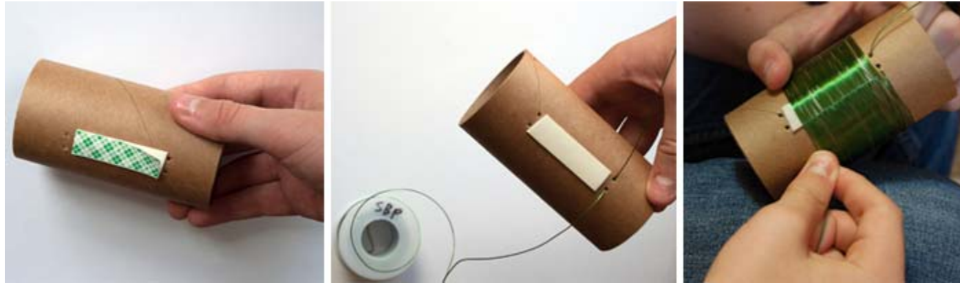
Figure 5. Steps for making the receiver coil for your AM radio receiver. Be sure to leave at least 12 inches of wire sticking out on both ends of the coil, after threading it through the holes.
