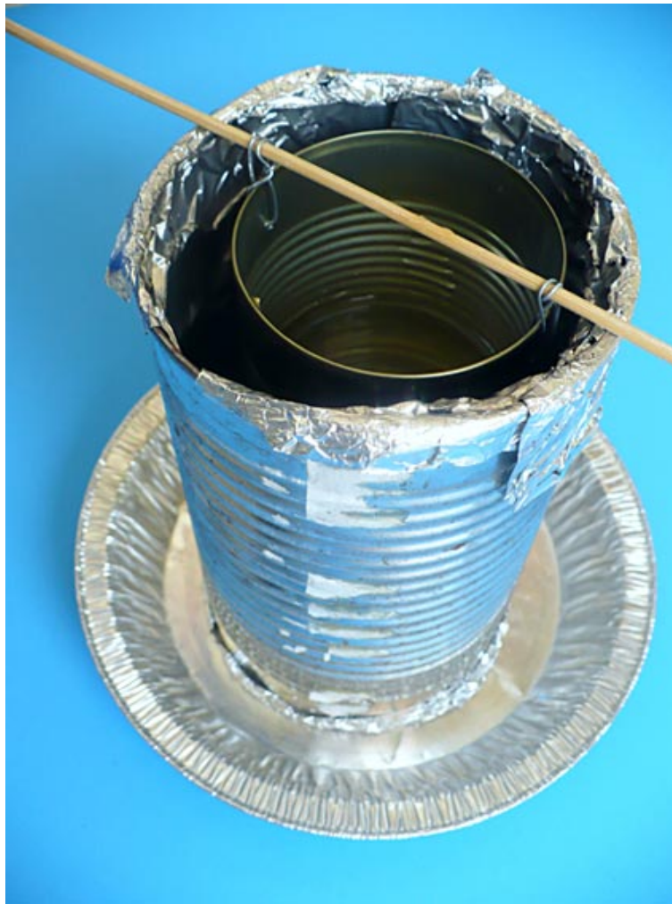
Figure 4. Top-down view of the assembled calorimeter.
