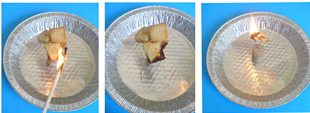
Figure 6. Some food items will need to be in flames before being put under the calorimeter.
