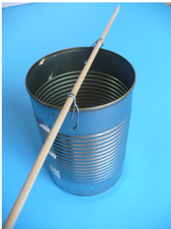
Figure 2. The rod can be attached on top of the small can with metal wire as shown here, or threaded through the holes.
