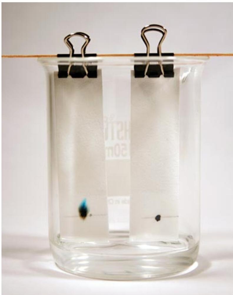
**Figure 5.** The edge of the chromatography strips should just barely touch the solvent. Remember to cover the top with plastic wrap so that the solvent does not evaporate.
