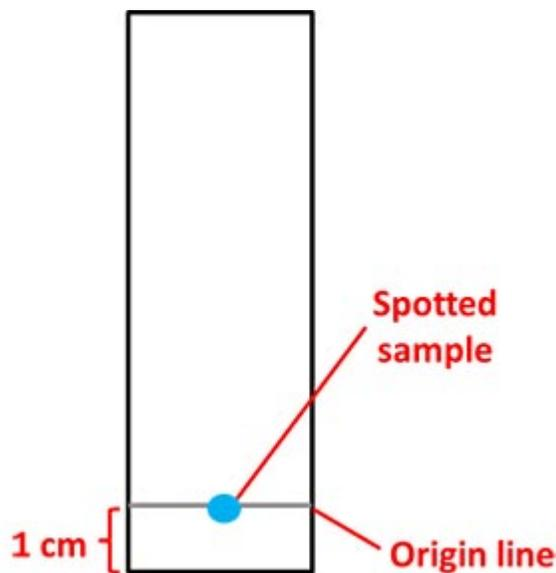
**Figure 3.** Each chromatography strip will have an origin line. The pen/marker ink to be tested will be spotted in the middle of the origin line.
