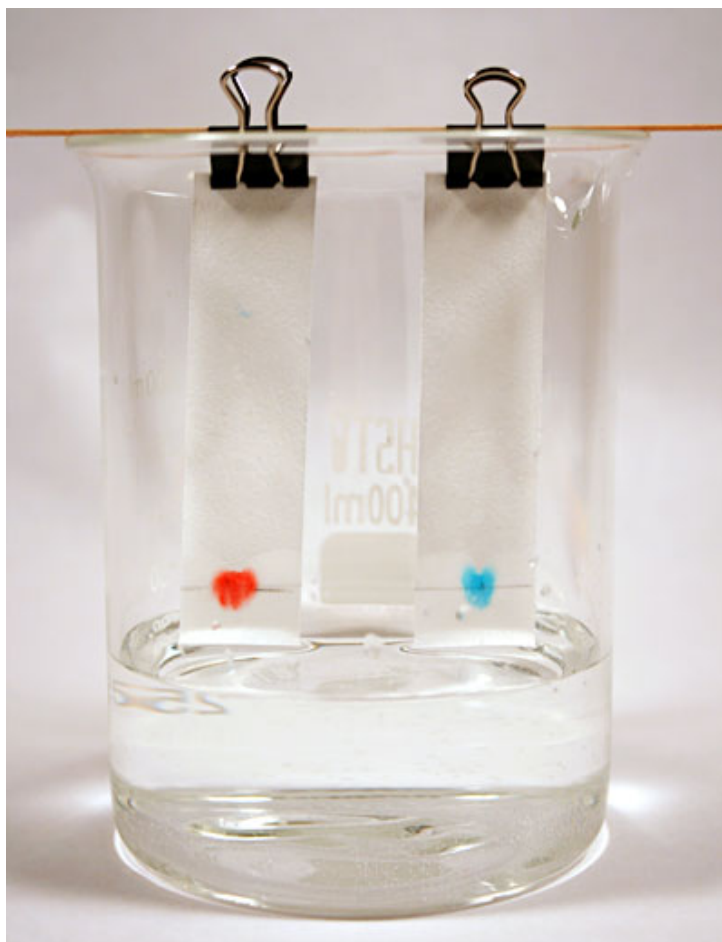
Figure 6. Your chromatography setup should look similar to this example. The edge of the chromatography strips should just barely touch the solvent.
