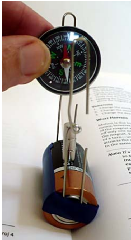
Figure 20. Figure showing how to determine the magnetic pole of the permanent magnet facing the electromagnet. If the red (north) end of the needle is pointing up, as shown in the figure, then the north end of the permanent magnet (and thus the magnetic field direction) is also facing up, and vice versa. This figure also shows from which angle to look at the motor when observing its direction of spin.
