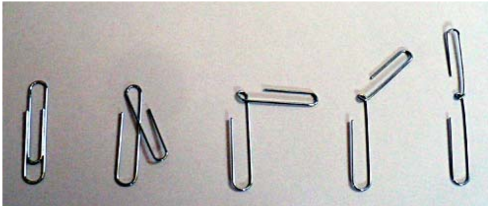
Figure 13. Step-by-step illustration of how to bend a paperclip (shown on the left) to create the axle support (on the right).
