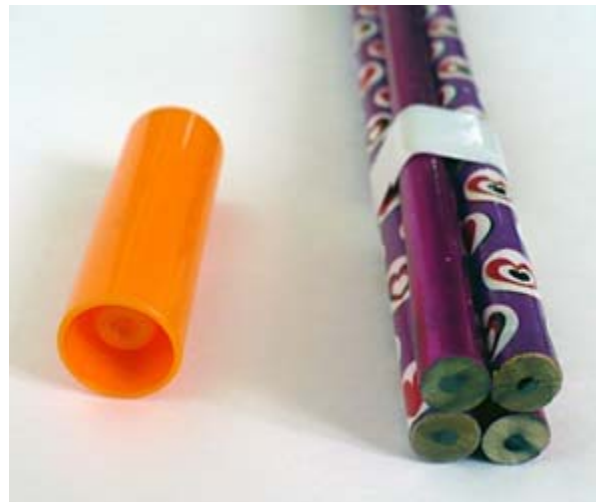
Figure 6. A felt-tip marker cap (left) or four pencils taped together (right) can be used to help neatly coil magnetic wire.
