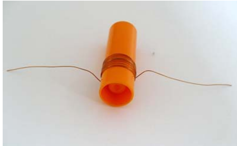
Figure 7. A coil (or electromagnet) is created by coiling magnetic wire 10\frac{1}{2} times neatly around a cylinder. Note 1.6 inches (4 cm) of wire is left free on each end to create the axles.
