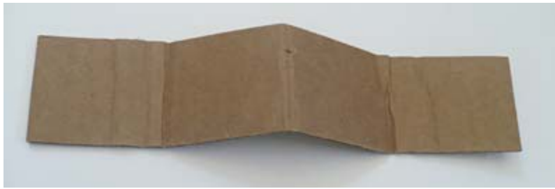
Figure 5. Pieces of corrugated cardboard that are folded in a V shape with flaps will help support the axle of the tool to help wind the iron cores.
