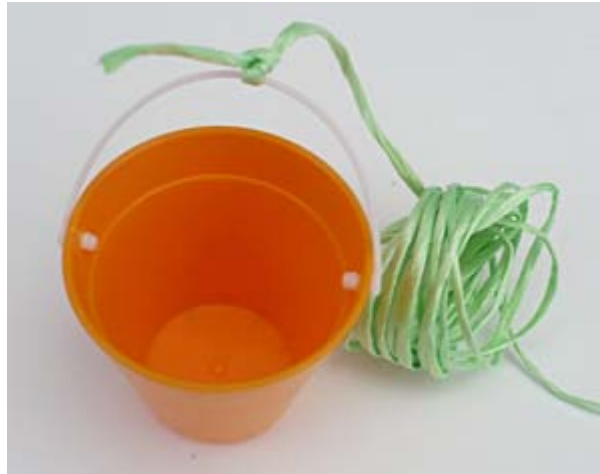
Figure 16. A cup or bucket hanging from a string will be used to create reproducible rotations of the generator's shaft.
