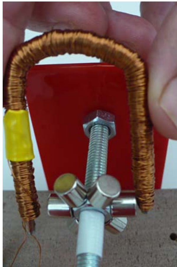
Figure 14. Shape the coil so the rotor fits inside the U shape, leaving just enough space to let it turn easily. Note: The magnets might pull the U shape toward it.
