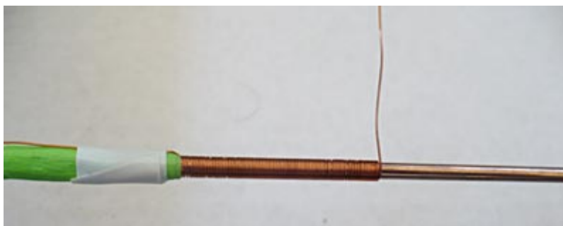
Figure 7. Loops of magnet wire placed neatly, one next to the other, around an iron core starting at a connection of the iron core with the L shape. The green masking tape holds the core and the L shape together to form the axle; the white tape holds the start lead in place.
