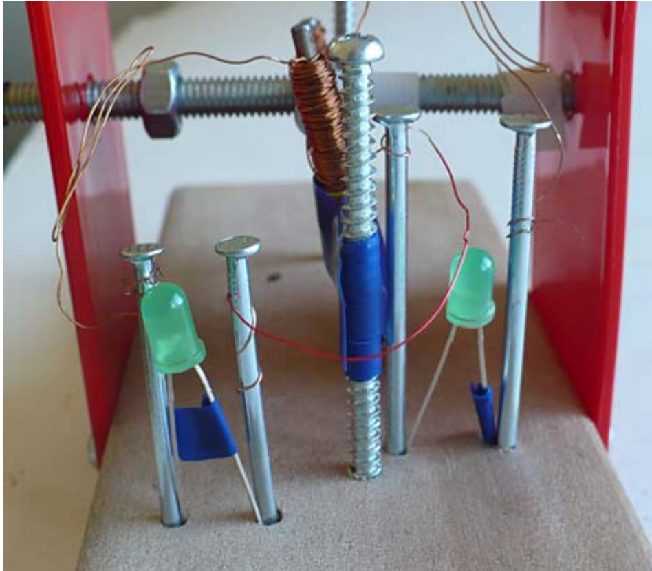
Figure 21. Two LEDs connected in series using two nails and an extra piece of wire. Note that the long (flagged) leg of one LED is connected to the short (unflagged) leg of the other LED.
