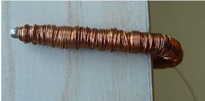
Figure 13. A straight coil is bent into a U-shaped coil at the edge of a table with the force of your hand.
