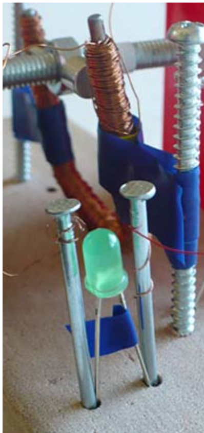
Figure 15. Electrical connections between the coil leads and an LED are created using two nails.
