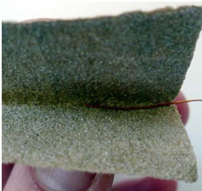
Figure 8. A "sandpaper sandwich" is used to remove the insulation from the ends of the magnet wire.
