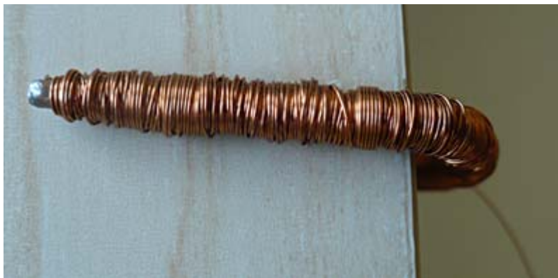
Figure 11. A straight coil is bent into a U-shaped coil at the edge of a table with the force of your hand.
