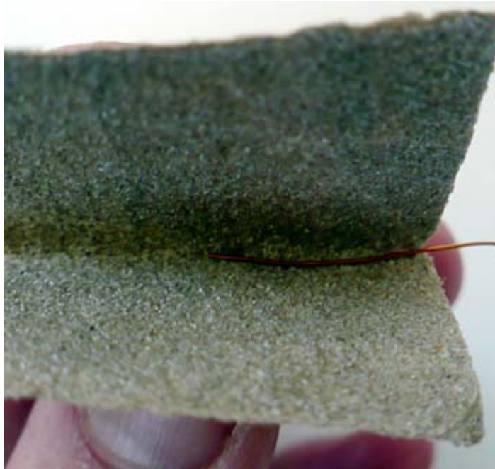
Figure 10. A "sandpaper sandwich" is used to remove the insulation from the ends of the magnet wire.
