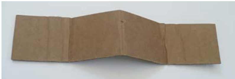
Figure 7. Pieces of corrugated cardboard that are folded in a V shape with flaps will help support the axle of the tool to help wind the iron cores.
