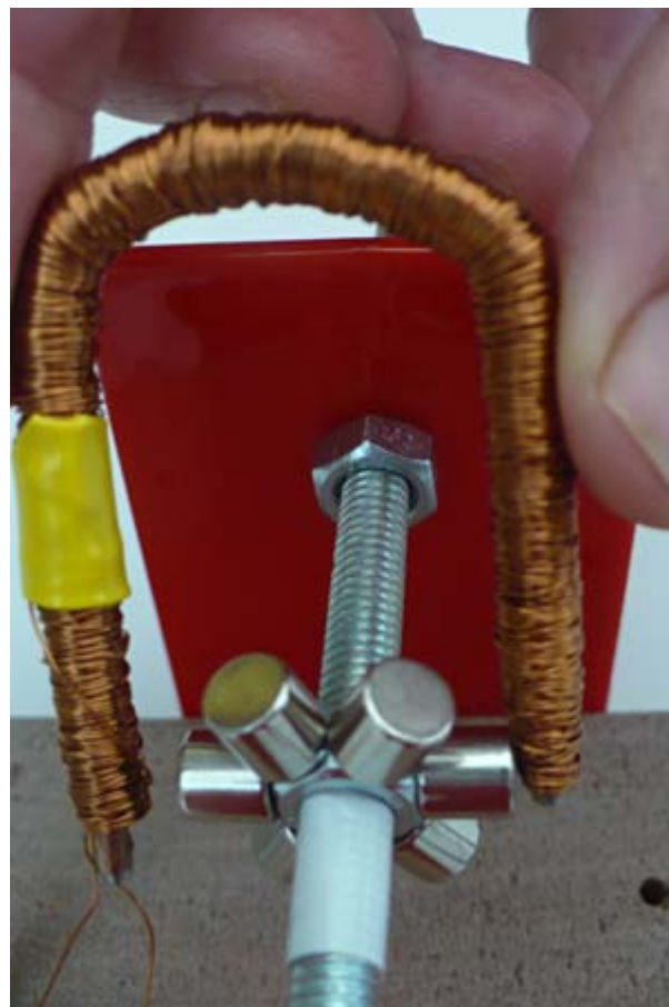
Figure 18. Shape the coil so the rotor fits inside the U shape, leaving just enough space to let it turn easily. Note: The magnets might pull the U shape toward it.
