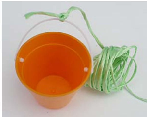
Figure 20. A cup or bucket hanging from a string will be used to create reproducible rotations of the generator's shaft.
