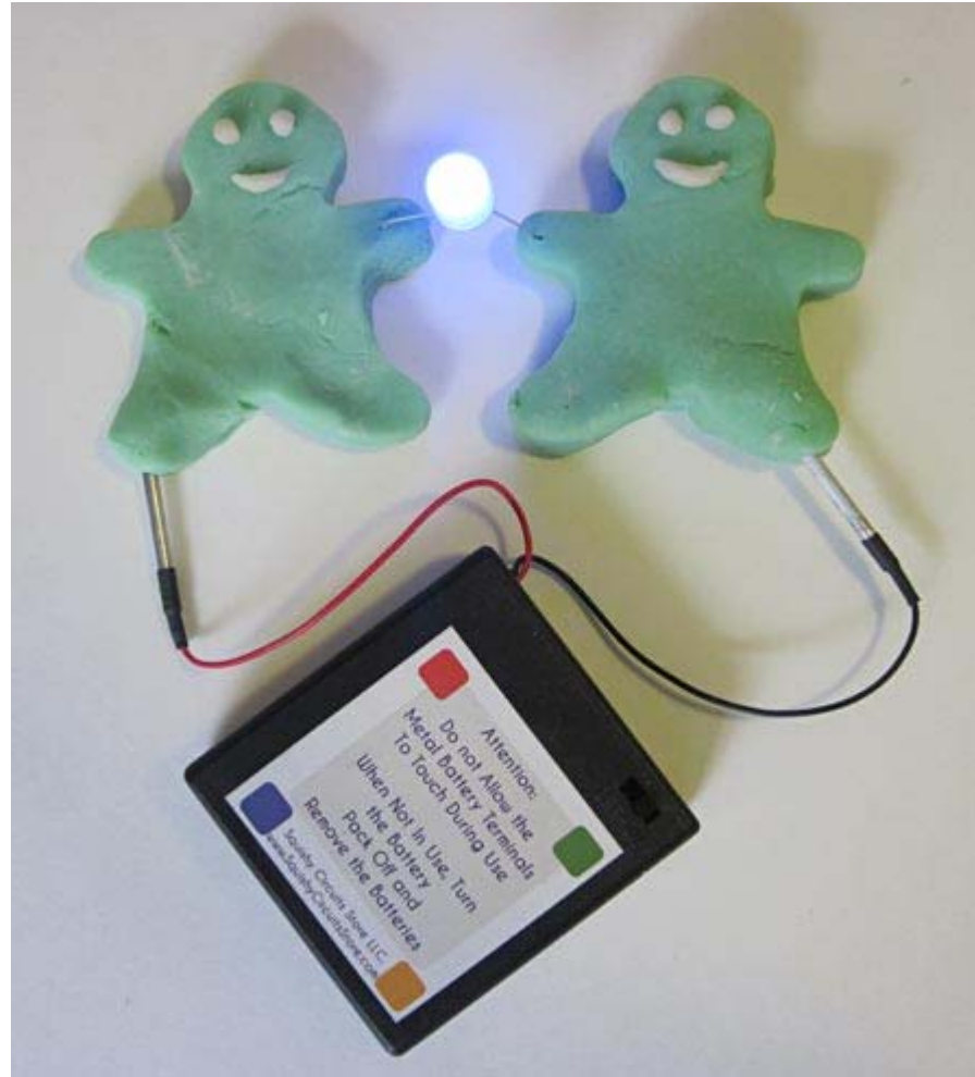
Figure 6. The shape of the Play-Doh pieces does not matter when connecting LEDs; as long as there is a closed circuit for electricity to flow (and no short circuit), the LED will still light up.
