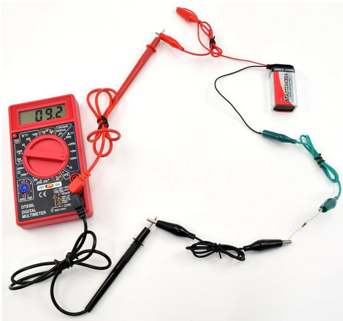
Figure 7. Setup for making sure the multimeter has a working fuse.
