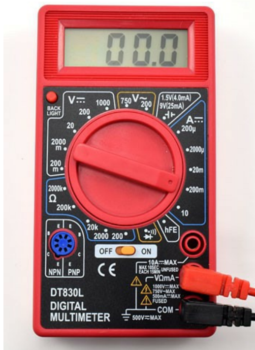
Figure 6. Multimeter dial set to the 200 milliamp (mA) range, represented by the "200m". Be careful not to get this mixed up with the "200m" on the other side of the dial. That setting is for measuring voltage, not current.
