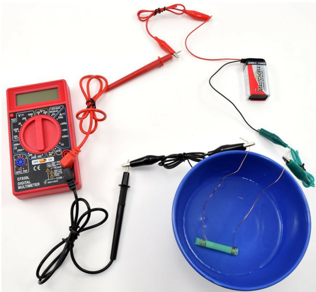
Figure 4. A picture of the completed conductance measuring circuit. The colors of the alligator clips do not matter.
