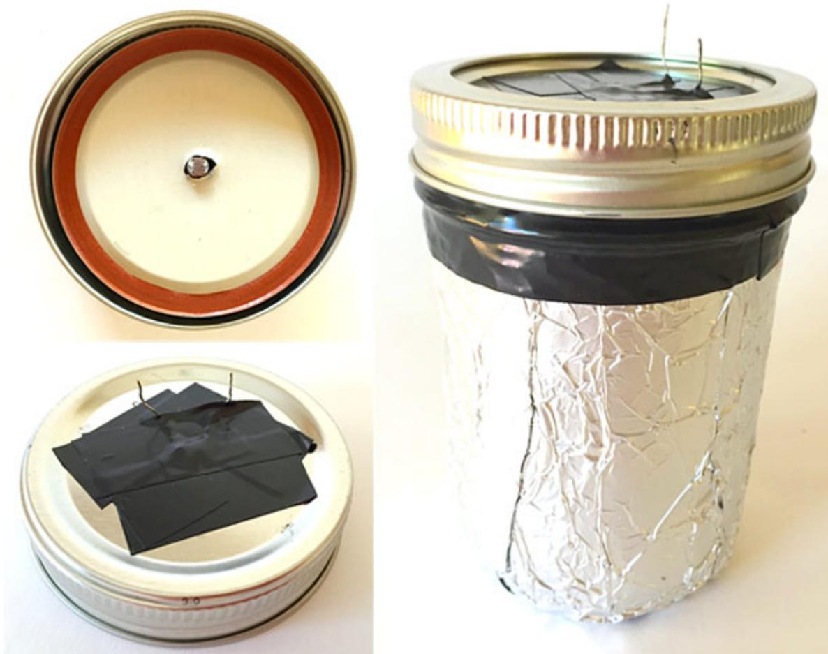
**Figure 3.** Preparing your light-measuring device by inserting the photoresistor into the lid of a glass jar (left) and wrapping the jar in aluminum foil (right). Make sure to seal all edges and protect the photoresistor from creating a short circuit
