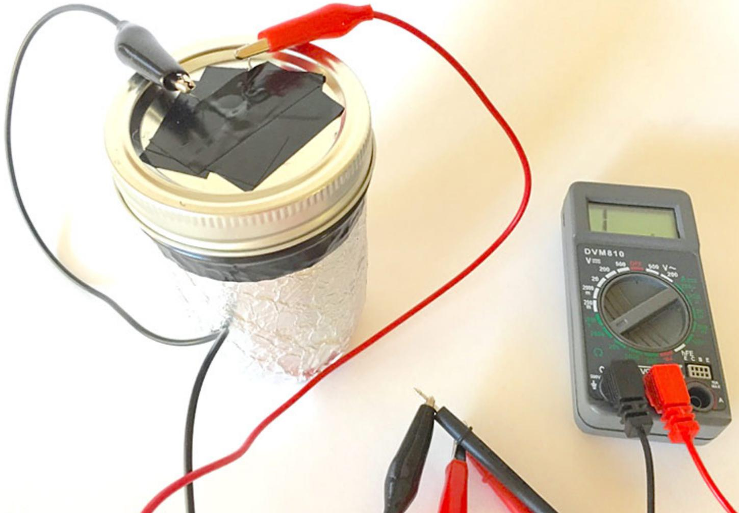
**Figure 3.** Setup of the light-measuring device for measuring the light intensity of glow-in-the-dark objects.
