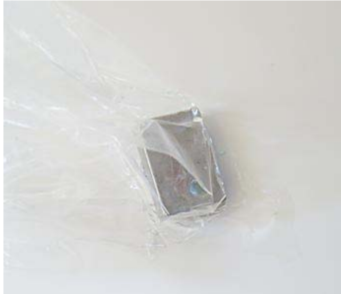
Figure 5. Place the neodymium magnet in the corner of the sandwich bag. It is now ready to pick up the magnetized oil spill in an oil cleanup procedure.
