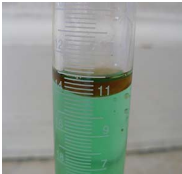
Figure 6. This close-up picture of a graduated cylinder can help determine the volume of oil left on the water. Make sure your camera is level with the oil fluid and markings on the cylinder are visible before taking a picture.
