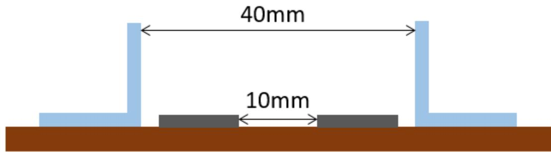
**Figure 4.** Cross-sectional view of the spacing for the magnet strips and plastic angle pieces.
