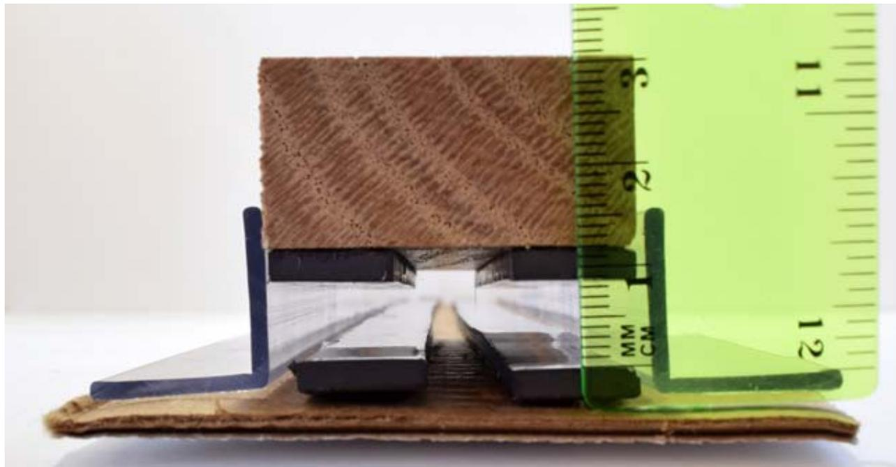
**Figure 7.** Use a ruler to measure the distance between the train and the track.
