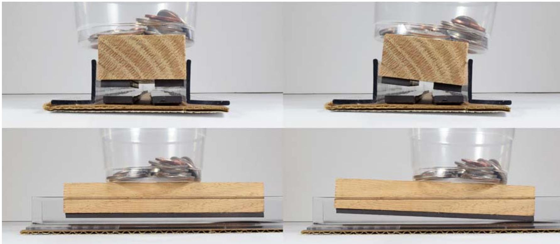
**Figure 9.** Check the train from both the front and the side to make sure it is still floating parallel to the track, as shown in the left two images. If the train is tilted, like in either of the right two images, then shift the location of the cup to balance the train.
