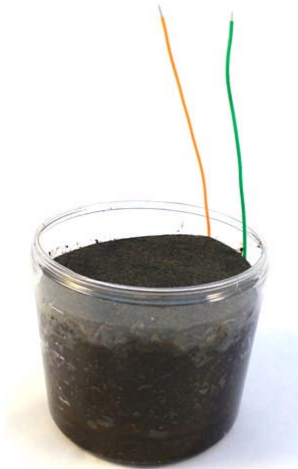
Figure 5. Add the cathode on top of the 5 cm of mud.
