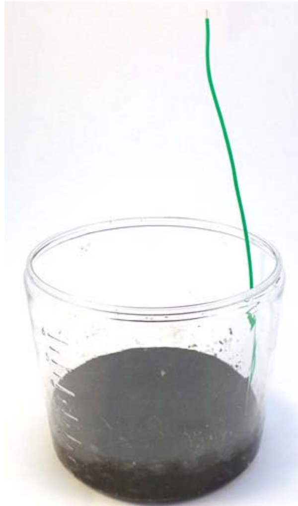
Figure 4. Place the anode on top of the 1 cm of mud.
