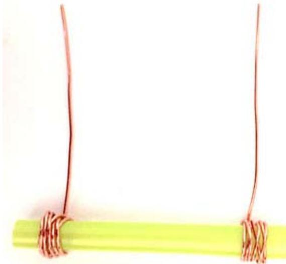
**Figure 6.** The conductivity sensor consists of a non-conducting core (a piece of disposable drinking straw) with copper wire wrapped around the ends. The ions in the solution complete the circuit, enabling current to flow between the copper wires.
