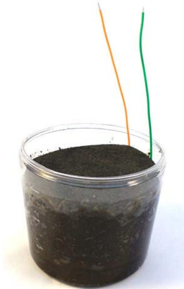
**Figure 4.** Add the cathode on top of the 5 cm of mud.
