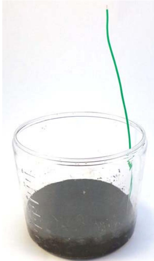
**Figure 3.** Place the anode on top of the 1 cm of mud.
