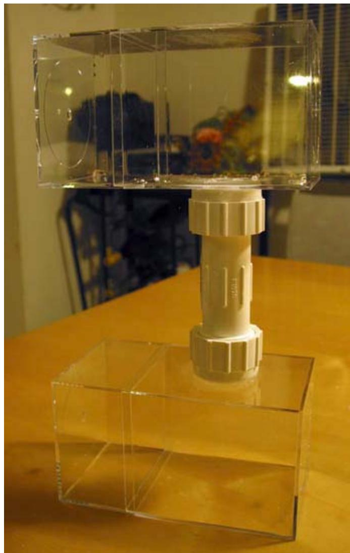
**Figure 4.** Aligning and cementing the second endcap and container.
