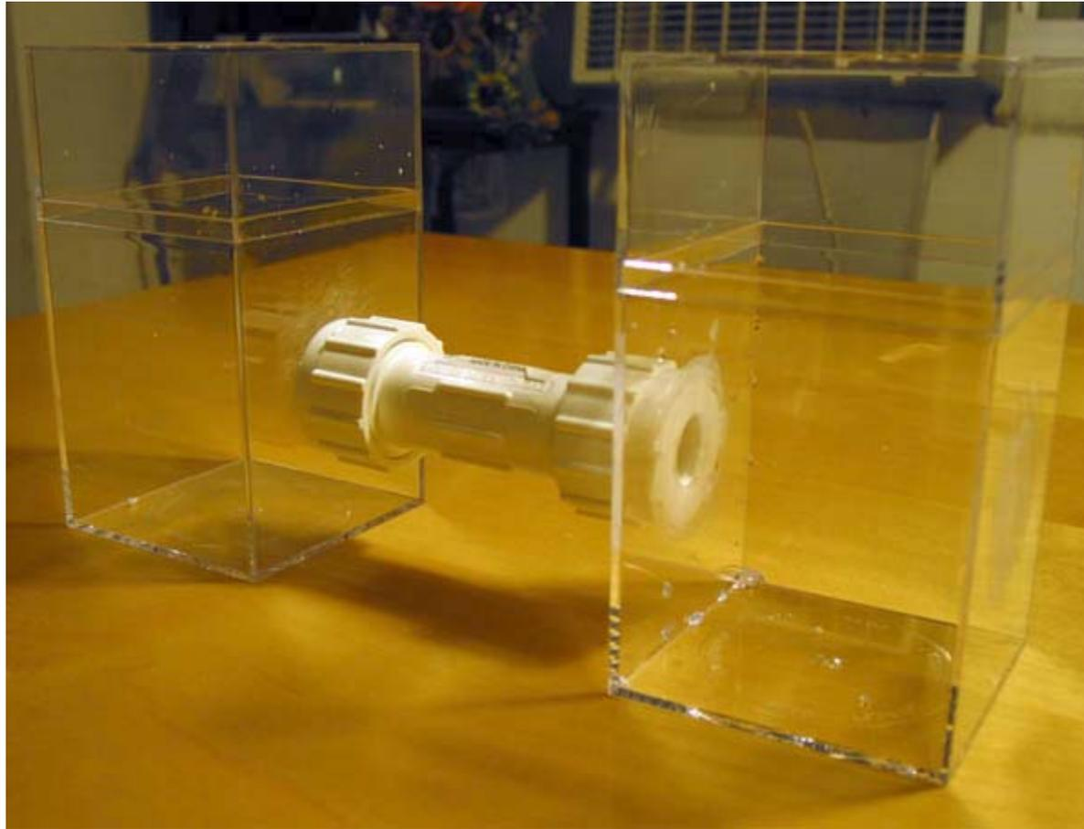
**Figure 5.** This is one set of a connected anode and cathode chamber.
