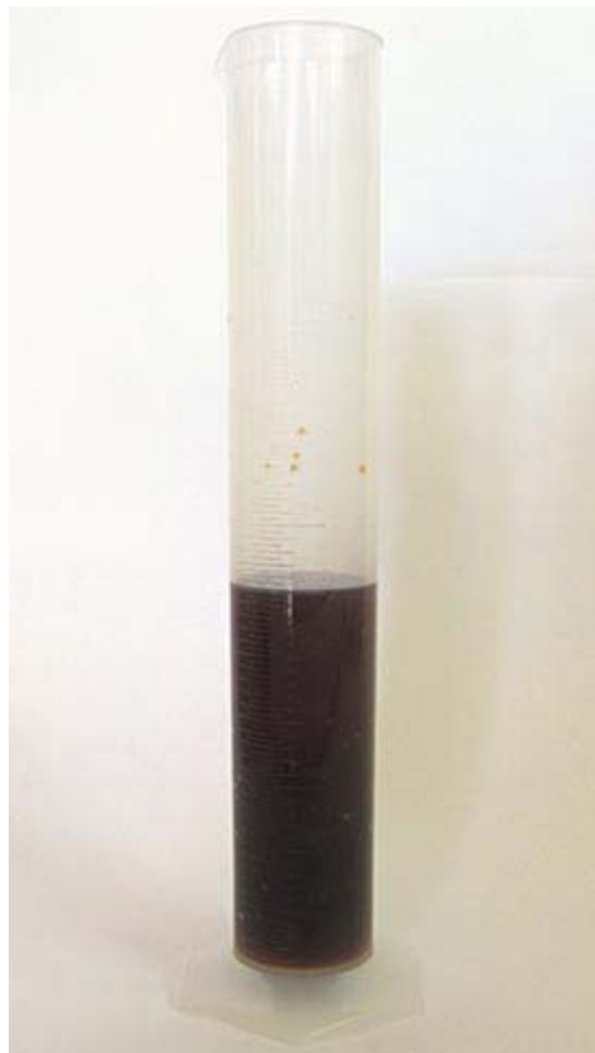
Figure 1. After adding the 30 mL of Lugol's iodine solution to the 500 mL graduated cylinder, add enough distilled water to bring the total fluid volume up to 300 mL.
