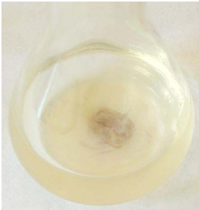
Figure 11. When you add a drop of iodine solution, you may see a temporary color change, as shown here (the dark blue swirls), that goes away when the iodine solution is mixed in the flask by swirling it.
