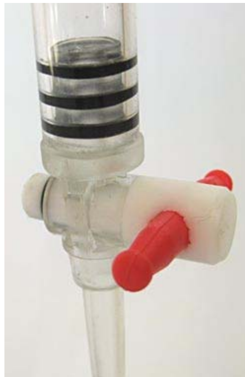
Figure 9. Make sure the buret is turned to the closed position, as shown here with the buret from the Science Buddies kit.
