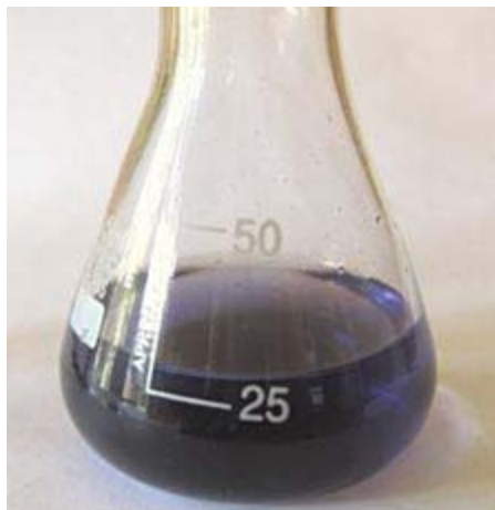
Figure 12. When the entire solution in the flask changes to a blue-black color that lasts for more than 20 seconds while swirling it, the titration is complete.
