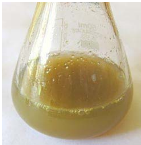
Figure 14. When the titration is complete with the orange juice sample, the entire orange juice sample will turn from orange to grayish brown in color, as shown here.
