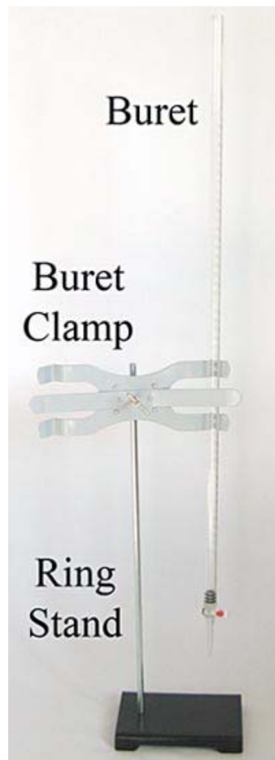
Figure 5. Assemble the ring stand, buret clamp, and buret, as shown here.
