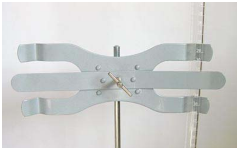
Figure 6. Carefully slide the buret into place between the prongs of the buret clamp.
