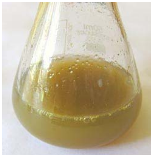
Figure 14. When the titration is complete with the orange juice sample, the entire orange juice sample will turn from orange to grayish brown in color, as shown here.
