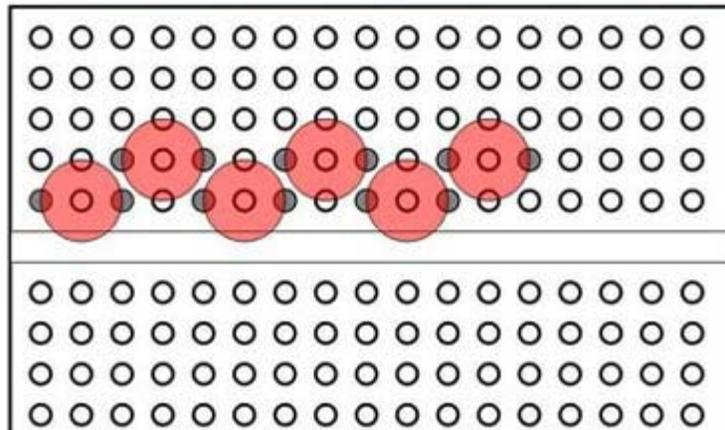
**Figure 8.** Arrange six LEDs in a staggered row on the breadboard, as shown here. (Top) A photograph of the actual breadboard. (Middle) A zoomed-in photo of the LED leads pressed into the breadboard holes. (Bottom) A top-down diagram of the breadboard showing the LED lights (red circles) and the holes to place the LED leads into (the small, solid gray circles). Remember to make sure all the *longer* LED leads are facing left, and all the *shorter* LED leads are facing right.
