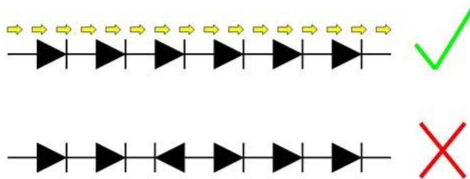
**Figure 9.** The triangle symbol with a line at the tip represents a single LED. When multiple LEDs are all connected facing the same direction, electrical current can flow through them. If just one LED is placed backwards, then electrical current cannot flow at all.
