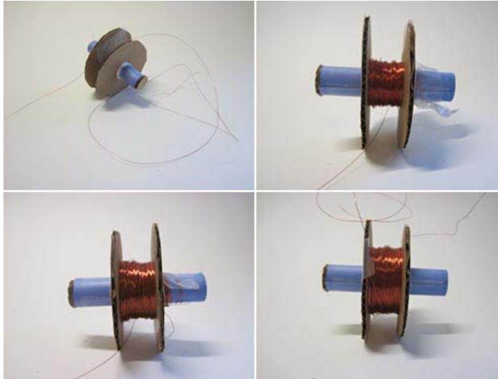
**Figure 7.** Carefully and tightly wrap the wire around the coil form for a total of approximately 1,500 wraps. This figure shows (top left) zero wraps, (top right) 500 wraps, (bottom left) 1,000 wraps, (bottom right) 1,500 wraps.
