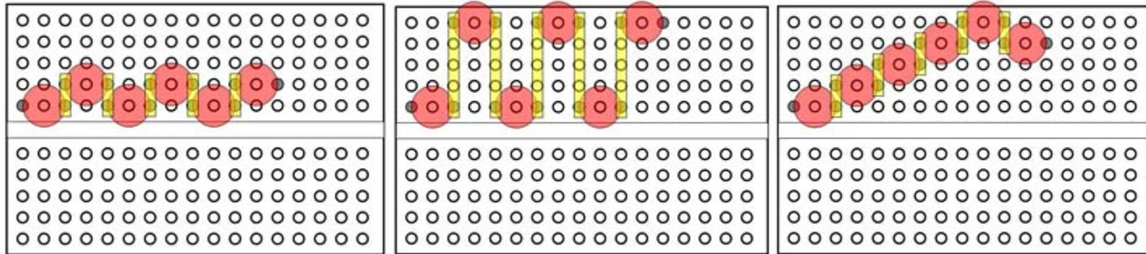
**Figure 11.** These three breadboard LED arrangements are all electrically equivalent. In each case, the leads of adjacent LEDs are connected through rows in the breadboard (highlighted by the yellow rectangles).
