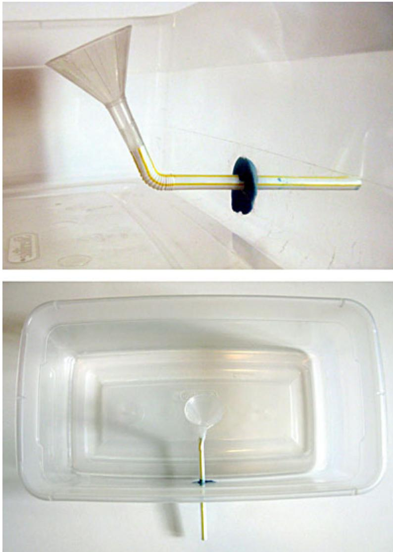
**Figure 3.** After putting the straw-funnel assembly in the hole in the container and securing it using some modeling clay, your setup should look similar to the one shown here. The top picture shows a close-up from the side and the bottom picture shows an overall view from above.
