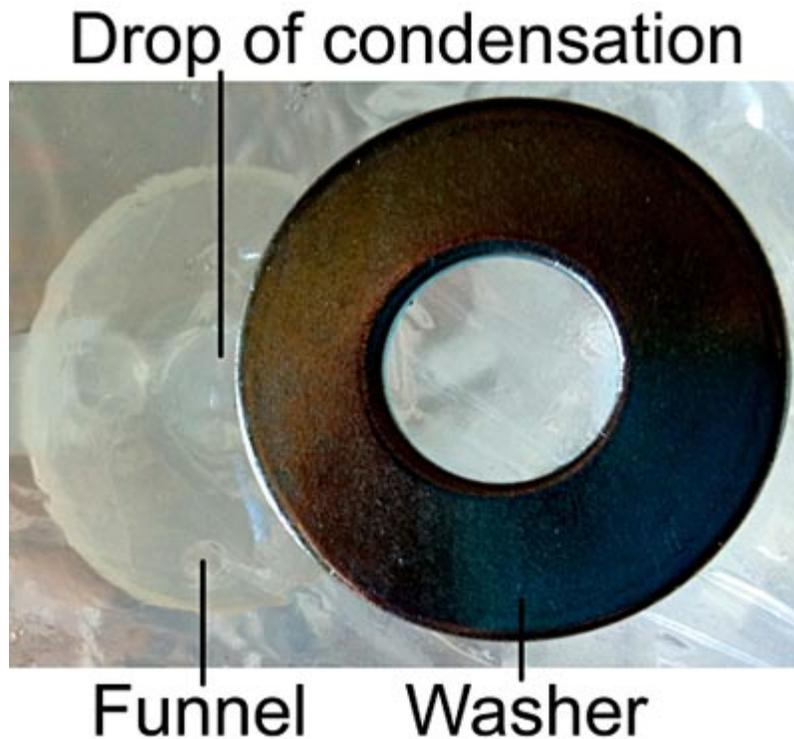
**Figure 7.** As shown in this close-up picture, you can arrange the washer so that its edge is the lowest point on the cling wrap and is positioned over the funnel, allowing condensation to drop into it.
