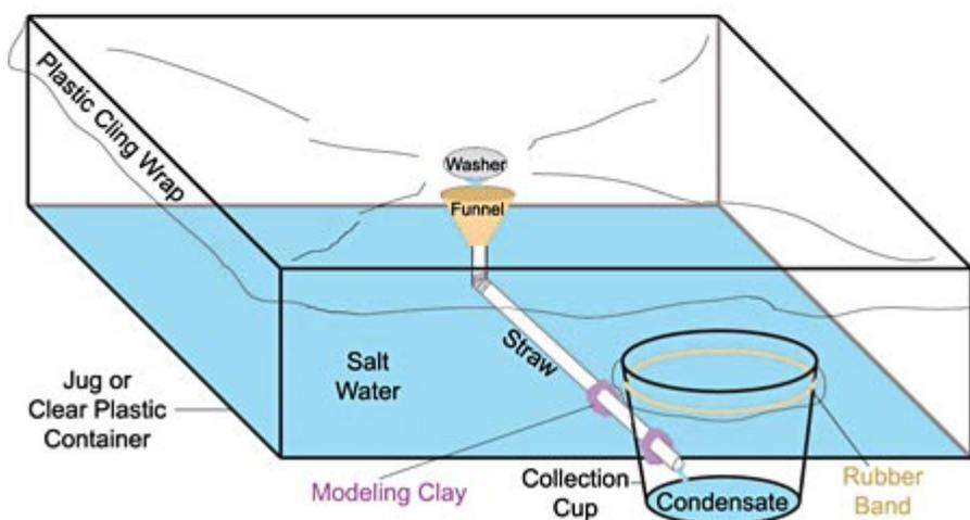
**Figure 6.** When your desalination devices are ready for testing, they should look similar to the one in the top picture (except yours should have black or white construction paper on the bottom). The diagram on the bottom shows what the desalination devices should look like during testing as condensation is collected. (The construction paper is not shown in the diagram.)
