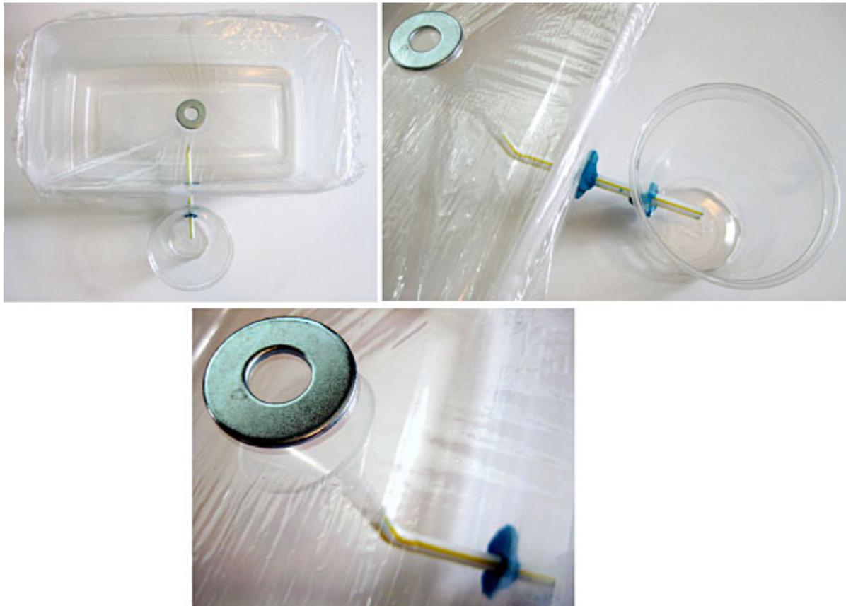
**Figure 4.** Place the washer on the cling wrap, right above the funnel. Make sure that the cling wrap is not so low that it is touching the funnel. The top left picture shows the entire setup at this point. The top right picture shows a close-up of the collection cup and washer. The bottom picture shows a close-up of just the washer and funnel.
