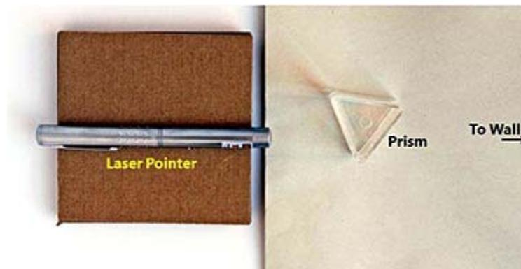
**Figure 7.** Photograph showing experimental setup for measuring the index of refraction of a liquid. The prism is a few centimeters in front of the laser pointer. The laser pointer is pointing perpendicular to a nearby wall.
