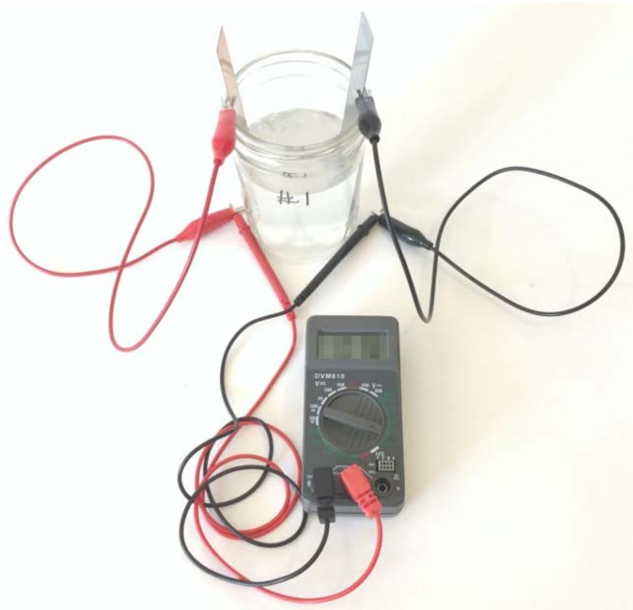
**Figure 5.** Setup for measuring the open-circuit voltage and short-circuit current of your zinc-air batteries. *Note:* The multimeter screen has been blurred in the image. We do not want to give away the data!
