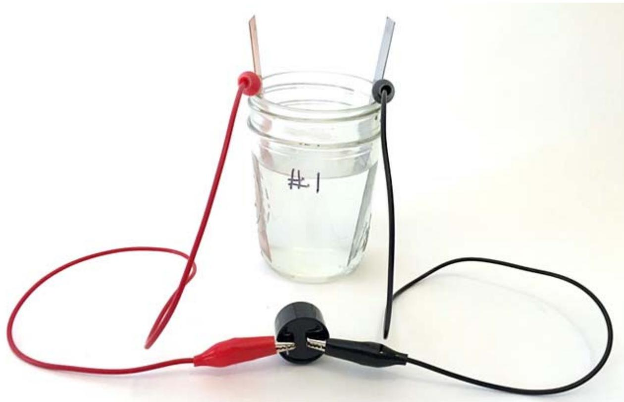
**Figure 4.** Alligator clips connected to the buzzer. **Note:** the buzzer shown in this picture has short metal pins, with one marked by a "+" sign for positive. Your buzzer may have longer red (positive) and black (negative) wires attached.
