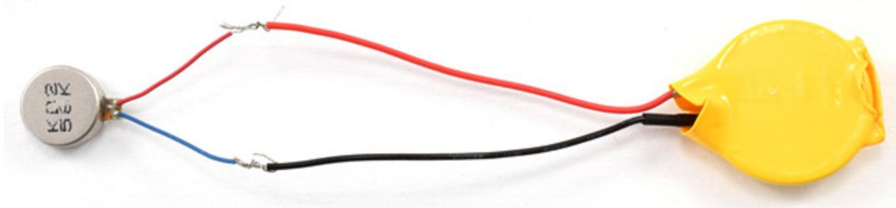
**Figure 2.** Motor (the gray circle on the left) and battery (the yellow circle on the right) wires connected to form a circuit.
