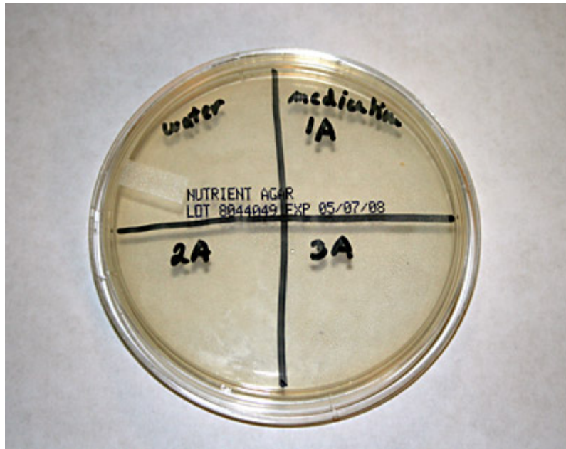
Figure 3. This photo shows how your agar plates should be divided into quadrants and labeled.
