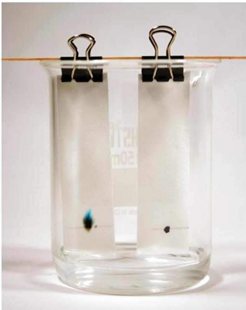
**Figure 6.** Your setup should look similar to this example. The end of the chromatography strip should just touch the alcohol. *Note:* This picture does not show chromatography strips with plant extract. The colors on your paper strips should look different.
