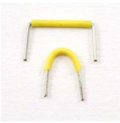
3. Some of the jumper wires in your kit might be longer than necessary. Bend them into U-shapes, as needed, to fit them into the breadboard.
