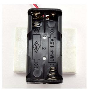
4. Mount the battery holder to the sticky tape, as shown. Make sure it is centered on the breadboard.
