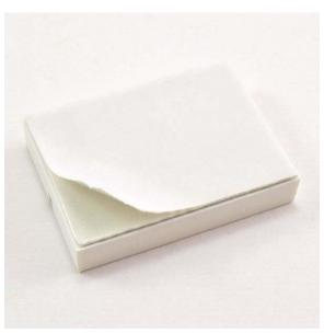
3. Peel the paper backing off the bottom of the breadboard to expose the sticky tape.
