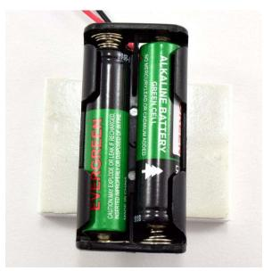
5. Insert the AAA batteries into the battery holder. Press the flat ends of the batteries up against the metal springs.
