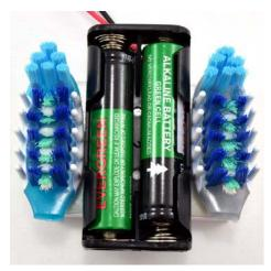
6. Attach the two toothbrush heads on either side of the battery holder. Make sure to mount them symmetrically.
