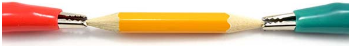
Figure 6. Connect red and green alligator clips to the graphite point at each end of a sharpened pencil.
