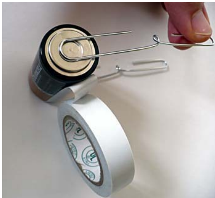
Figure 15. Secure the second paperclip to the battery with tape to complete the axle support.
