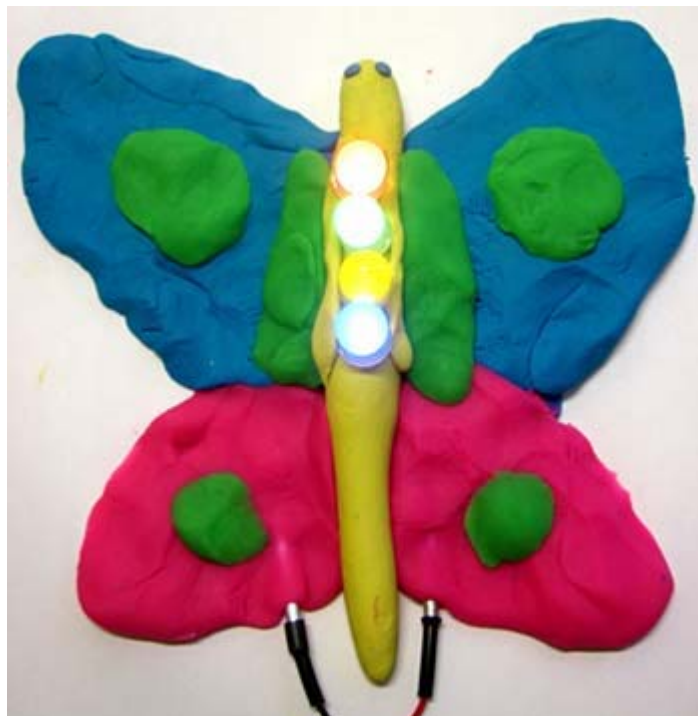
Figure 8. An example design with four LEDs in parallel. The wings of the butterfly are made from conductive Play-Doh and the body in the middle (yellow) is made from insulating modeling clay.
