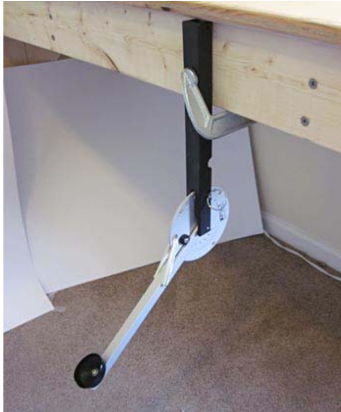
Figure 4. Catapult clamped to the bottom edge of a workbench.
