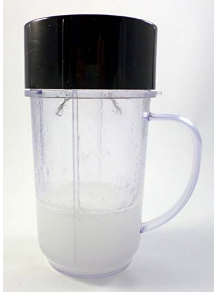
Figure 3. Blend the sodium alginate with the water until they make a smooth solution.
