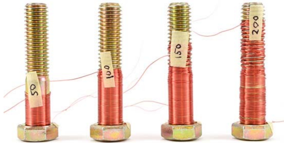
Figure 2. Four electromagnets with 50, 100, 150, and 200 turns of wire, respectively.
