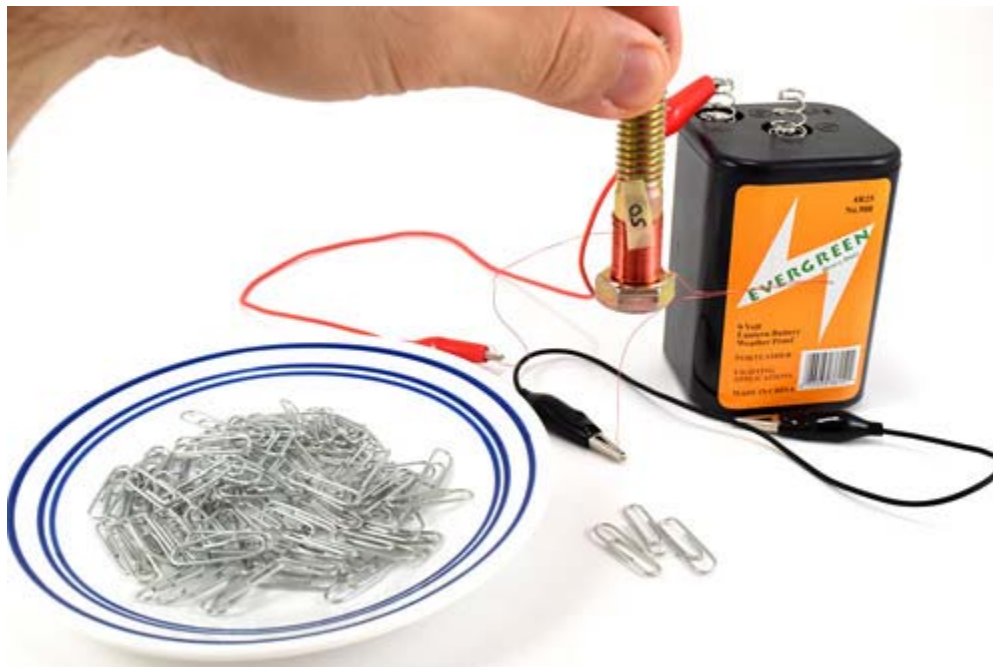
Figure 4. Lifting paper clips with the electromagnet.
