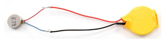
Figure 2. Motor (the gray circle on the left) and battery (the yellow circle on the right) wires connected to form a circuit.
