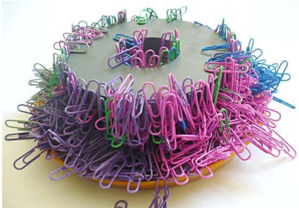
Figure 4. The magnet rests on a flat pile of paper clips that were originally placed as a flat pile on a plate or flat surface. The number of paper clips it picks up when removed is a measure of the strength of the magnet.
