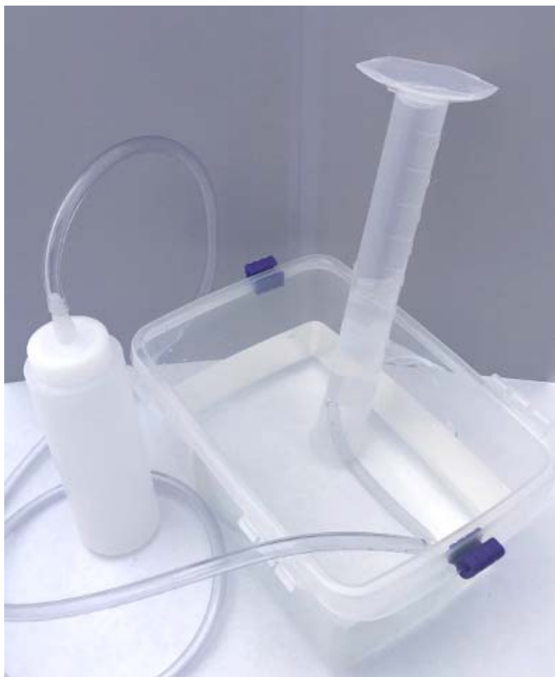
Figure 3. Picture of the inverted graduated cylinder gas collection apparatus.
