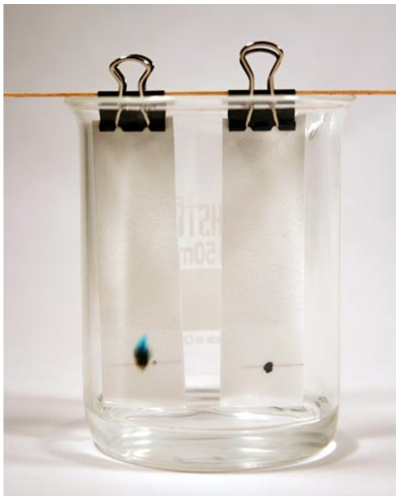
Figure 4. Your setup should look similar to this example. The end of the chromatography strip should just touch the alcohol. Note: This picture does not show chromatography strips with flower pigments. The colors on your paper strips should look different.
