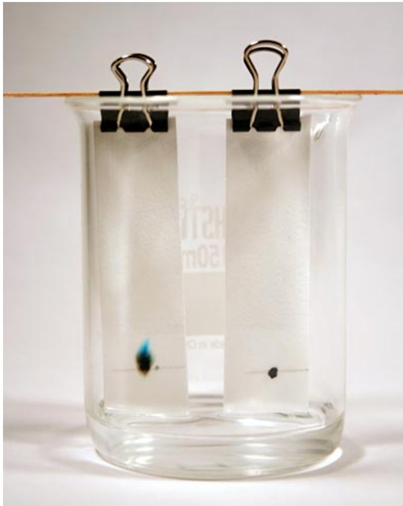
Figure 7. Your setup should look similar to this example. The end of the chromatography strip should just touch the acetone. Note: This picture does not show chromatography strips with plant extract. The colors on your paper strips should look different.
