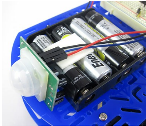
Figure 6. Mount the PIR sensor to the front of your robot using double-sided foam tape.
